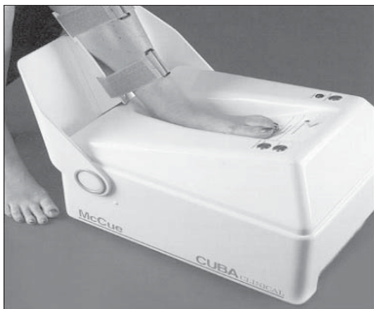
Fig. 1. Measuring BUA over the left heel using the CUBA machine.
